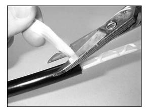
Figure 8 – Cut and remove the dielectric strength elements at the required length.
