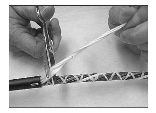
Figure 25 - Cut and remove the dielectric strength elements at the required length.
