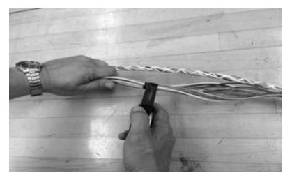
Figure 33 – Wrap a piece of vinyl tape around the outer buffer tubes to keep them in a bundle.
