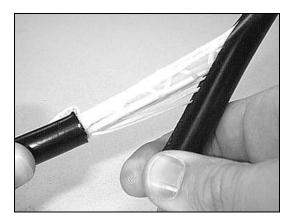
Figure 7 - Remove the outer jacket.
