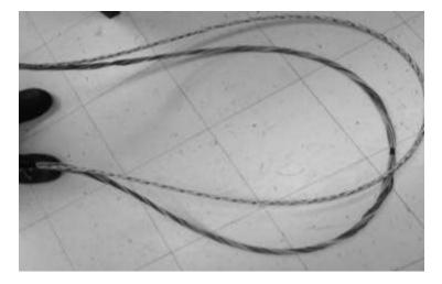
Figure 34 – Unwind the outer tube buffer layer from the inner layer.
