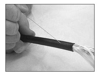
Figure 24 - Pull the ripcord to the marked length.
