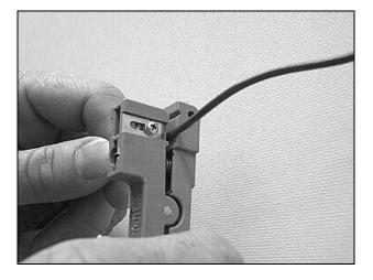
Figure 11A – Score the buffer tube with a buffer tube cutter.
