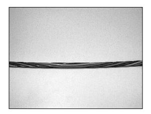
Figure 20 – Buffer tube reversal point.
