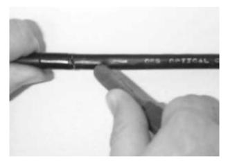
Figure 16 - Make a longitudinal cut between the two ring cuts.
