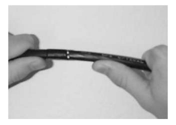
Figure 23 - Flex the cable jacket to separate at the score mark.
