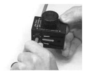
Figure 11B – Use a Quick Split RT tool to score *AccuTube* buffer tubes.
