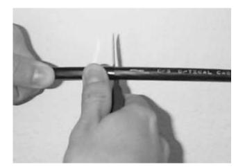
Figure 14 – Ring cut the cable jacket.
