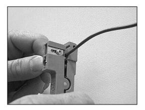
Figure 29 – Ring cut the buffer tube.
