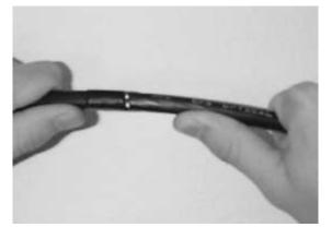
Figure 3 – Flex and separate the cable jacket.
