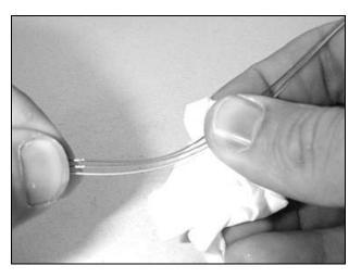
Figure 12 – Clean the optical fibers.
