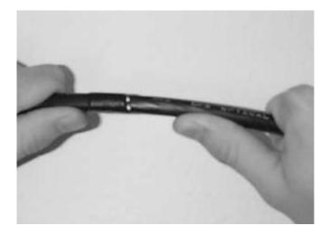
Figure 15 - Flex the cable jacket to separate it at the score mark.
