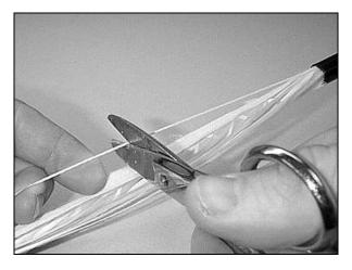
Figure 18 - Cut the ripcord in the center of the exposed length.
