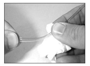
Figure 30 - Clean the optical fibers.
