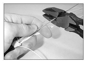
Figure 28 - Cut the central member to the required length.
